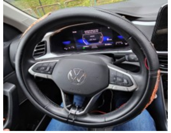
Fig. 2. Smart Steering wheel cover installed on a test vehicle
